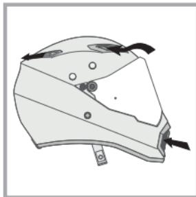
The front air intakes and the chin guard intakes can be opened and closed as desired, while the rear extractors, the only object of which is to allow air to escape from inside the helmet, are always open, allowing air to escape at a rate proportional to the increase of the travelling speed.
