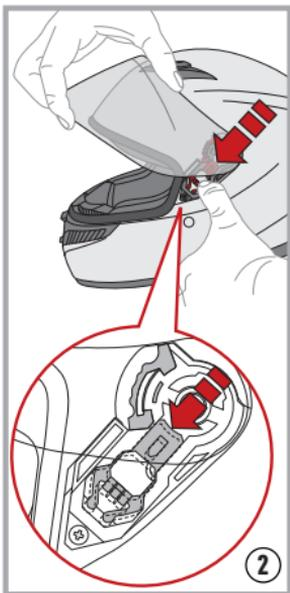
To fit the visor, start on one side of the helmet with the visor fully raised and insert the upper catch into its seating on the mechanism base ③.
